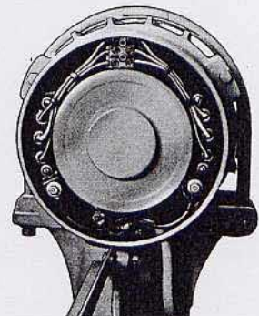
End view of generator with cover removed showing diodes and output terminals.
